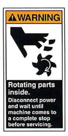
ALWAYS turn OFF the engine, wait five (5) minutes to make certain the flywheel and all moving parts have come to a complete stop and cool, and then disconnect the spark plug wires before servicing the machine. (#091-0381)
